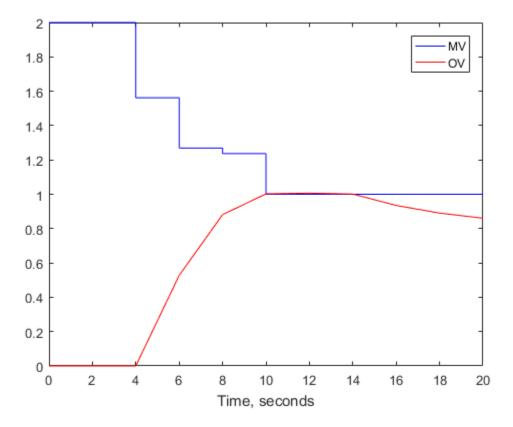
From the plot, you can observe that the original MV upper bound is active until t = 4. After the input delay of 4 seconds, the output variable (OV) moves smoothly to its new target of r = 1. reaching the target at t = 10. The new MV bound imposed at t = 10 becomes avtive immediately. This forces the OV below its target, after the input delay elapses.
